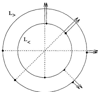
Fig. 5. The paths of the radial electron waves created by photoabsorption at the cluster edge. The different symbols for the point of creation indicate the four possible combinations which lead to interference with a respective path difference shown dashed.
