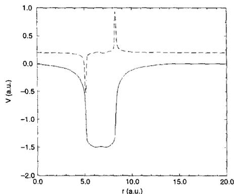
Fig. 2. The jellium potential for  $C_{60}$  from [9] (solid), and its derivative  $dV(r)/dr$  (dashed) entering the dipole operator of Eq. (1).
