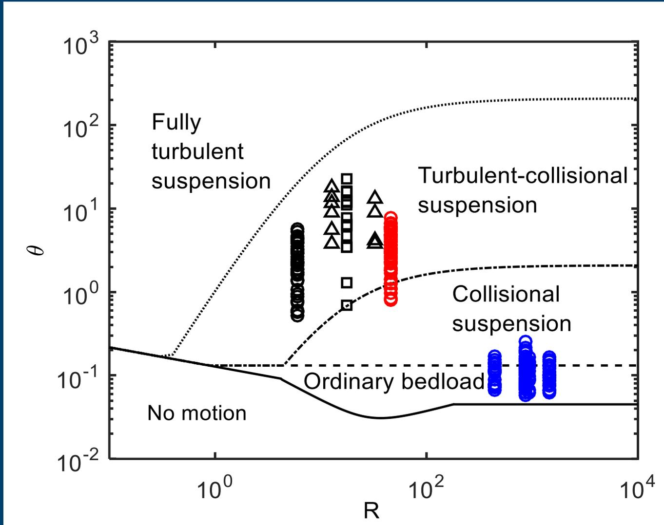
Steady, inclined, collisional sediment transport over an erodible bed in a turbulent fluid (Berzi and Fraccarollo, PHF 2013)
