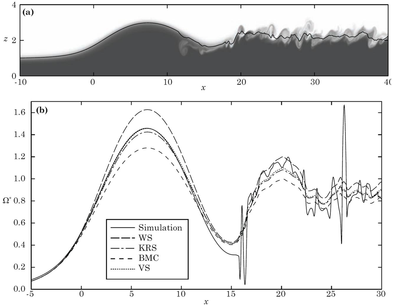
*Where the flow is approximately steady-state, the new circulation model yields the closest agreement with the DNS simulations*
