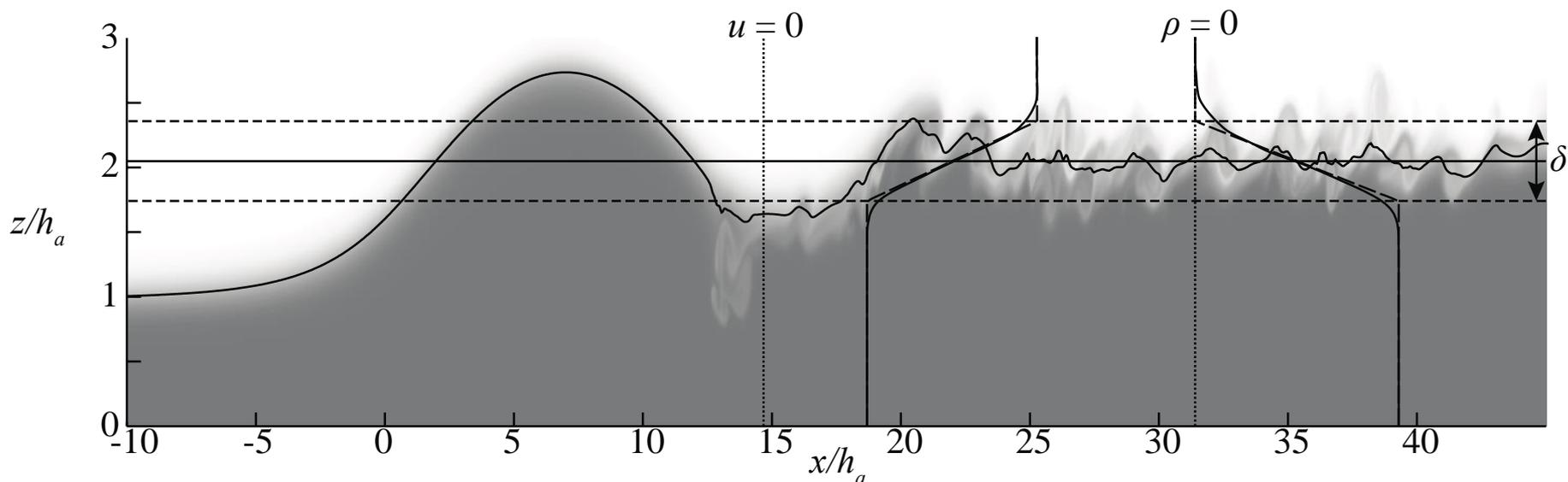
*Approximate velocity and density profiles by linear functions over mixing layer of thickness  $\delta$  :*
