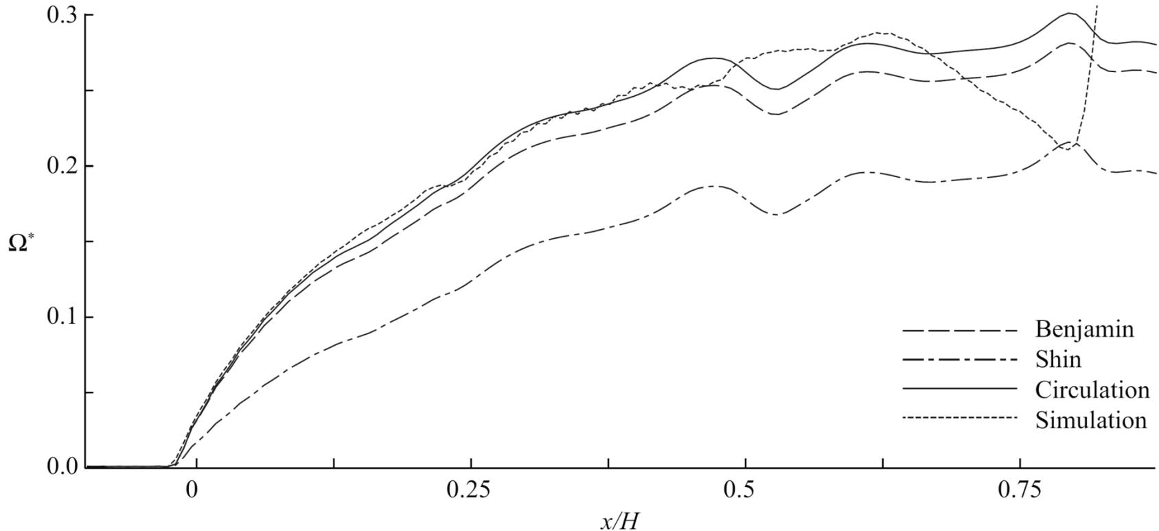
*Where the flow is approximately steady-state (near the current front), the new circulation model yields the closest agreement with the DNS simulations*
