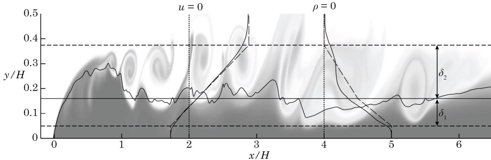
*Approximate velocity and density profiles by linear functions over mixing layer of thickness  $\delta_1$  and  $\delta_2$  :*
