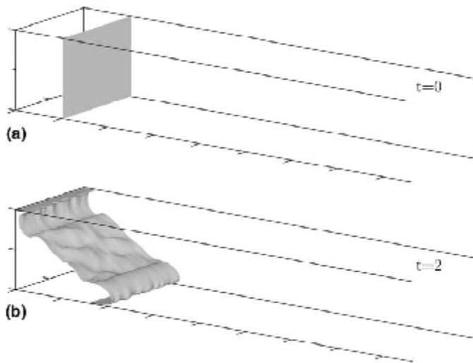
*Model problem: Lock-exchange gravity current*
