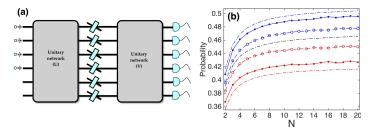
Panel (a): a lossy *M*-port A = UDV as a unitary 2*M*-port, where the beamsplitters have the transmission coefficients  $\eta_1, \ldots, \eta_M$  and  $D = \text{diag}(\sqrt{\eta_1}, \ldots, \sqrt{\eta_M})$ . Panel (b): the average survival probability of *N* indistinguishable bosons (above the middle dash-dot line) and fermions (below the middle dash-dot line) for M = 4N and m = 3 lossy channels with  $\eta_{1,2,3} = 0.1$  (dots) and  $\eta_{1,2,3} = 0.3$  (open circles).
