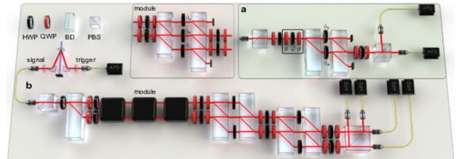
Figure 1: **Single-photon interferometer** for the nonunitary dynamics of (a) a single-qubit  $\mathcal{PT}$ -symmetric system and (b) a four-state qudit (consisting of spatial and polarisational degrees of freedom) for realising a higher-order exceptional point.
