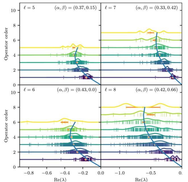
Figure 2: Extracted relaxation rates of  $m$ -local (operator order  $m$ ) Pauli string observables on  $\ell$  qubit subsets of `ibmq_16_melbourne`. The colored curves show distributions of the timescales, orange dots show the average relaxation rate. The theoretical prediction is a quadratic dependence on  $m$ , shown by blue curves. Figure from Ref. [6].
