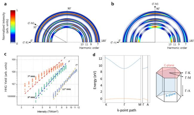
Figure 2: (a) Experimentally measured high harmonic spectra obtained by rotating the laser polarization direction in the C-plane, leading to the expected six-fold symmetry; (b) Measured high harmonic spectra from rotating laser polarization in the A-plane; (c) Experimental high harmonic yield plotted on a log-log scale for 7th (red), 9th (blue) and 11th (orange) order harmonics; (d) Sketch of the band structure of a sapphire crystal with the highest valence band and the lowest conduction band.
