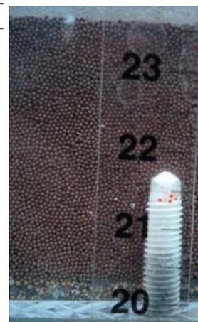
$\rho_s = 0.98 \text{ kg/m}^3$     $d = 0.45 \text{ mm}$     $\phi = 21^\circ$     $e = 0.75$     $\mu_w = 0.31$
