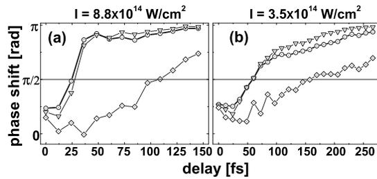
FIG. 4. Phase shift of the CM oscillation of quasifree electrons with respect to the driving field taken at the maximum of the second pulse as a function of delay between pulses. The phase shift of all quasifree electrons ( $\circ$ ), of quasifree electrons in the helium shell only ( $\nabla$ ) and in the xenon core ( $\diamond$ ) only is shown for  $\text{Xe}_{100} @ \text{He}_{500}$ .
