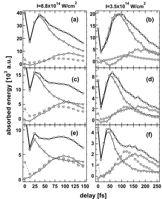
FIG. 3. Absorbed energy as a function of delay between pump and probe pulse for  $\text{Xe}_{100}@\text{He}_N$  ( $\circ$ ), for xenon atoms fixed ( $\nabla$ ), for bare  $\text{Xe}_{100}$  clusters ( $\square$ , dotted line) and finally, the difference in energy absorption for helium-embedded xenon clusters with moving and fixed xenon atoms ( $\diamond$ ). The panels (a) and (b) are for  $N=1000$  helium atoms, (c) and (d) for  $N=500$  and (e) and (f) for  $N=300$ , respectively.
