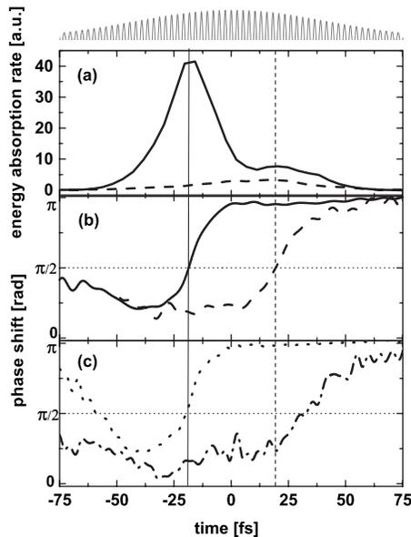
FIG. 2. Energy absorption rate (a), and phase shift of CM oscillations of the quasifree electrons with respect to laser field (b) for  $\text{Xe}_{100}@\text{He}_{1000}$  (solid) and  $\text{Xe}_{100}$  (dashed), respectively. Phase shifts for the embedded system  $\text{Xe}_{100}@\text{He}_{1000}$  (c) from electrons in the helium shell (dotted) and in the xenon core (dashed-dotted) only. Laser pulse (top) as in Fig. 1.
