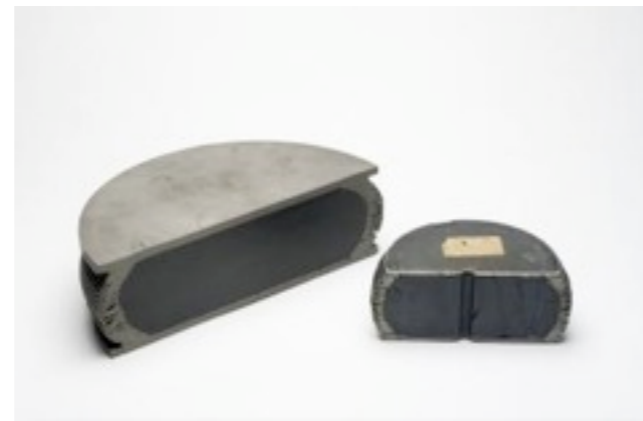
Waste forms - Synroc/ Oxide Ceramics
