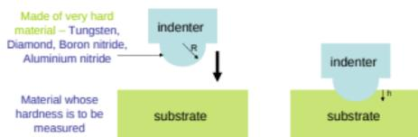
Measured quantities:- indentation load ( $P$ ), indentation depth ( $h$ )
