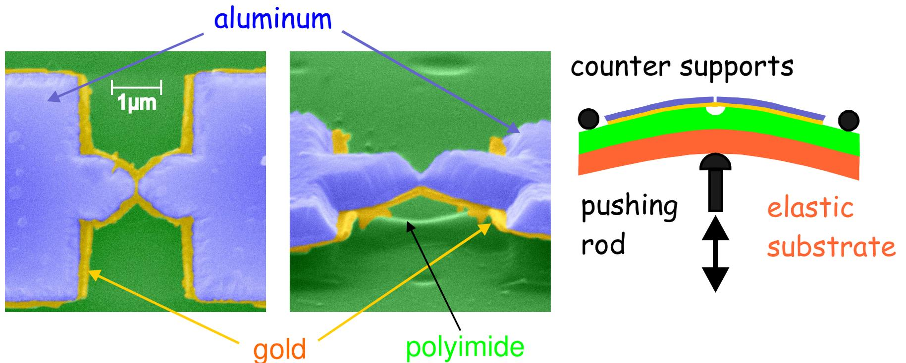
thickness of **aluminum** leads  $\sim 400$  nm
