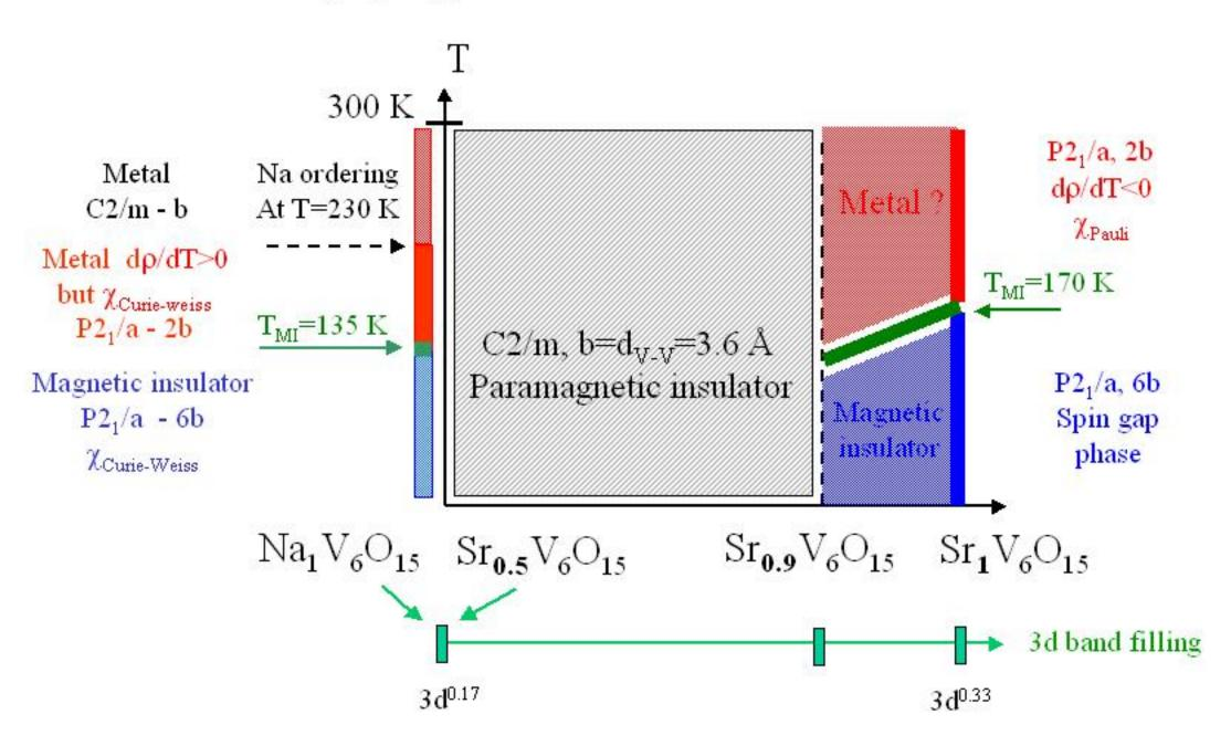
→ The MIT has been investigated by ARPES both as function of doping In  $Sr_xV_6O_{15}$  and as function of temperature in  $Sr_1V_6O_{15}$  and  $NaV_6O_{15}$ .
