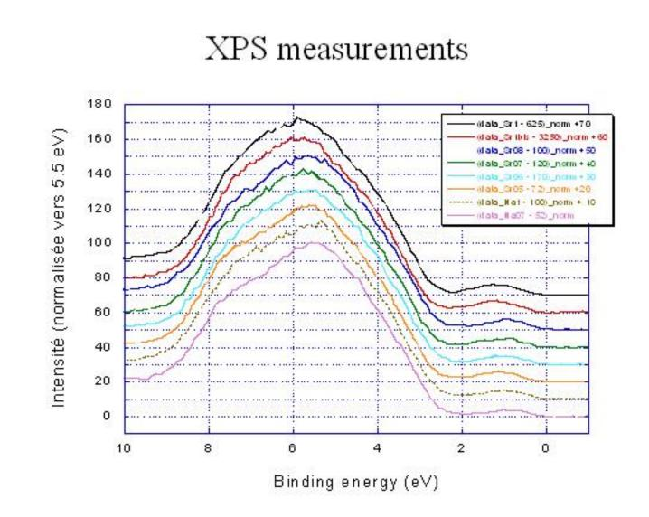
The position of the V<sub>3d</sub> incoherent peak (partially) follows the 3d band filling: E=1.24 eV in the case of  $Sr_{0.5}V_6O_{15}$  and  $NaV_6O_{15}$  which have the same filling  $(3d^{0.17})$  and E=1.44 eV for  $Sr_1V_6O_{15}$   $(3d^{0.33})$ . This is corroborated by XPS measurements suggesting that these measurements are bulk-like!
