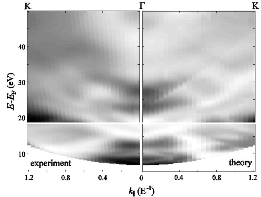
Electron transmission as a function of electron incidence angle and energy
