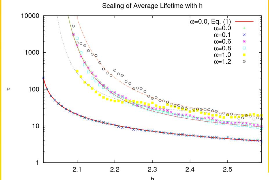
For zero coupling, the lifetime of the system follows the analytic solution Eq. (1). In the coupled case, the average lifetime grows to significantly larger times, following the scaling law Eq. (2).
