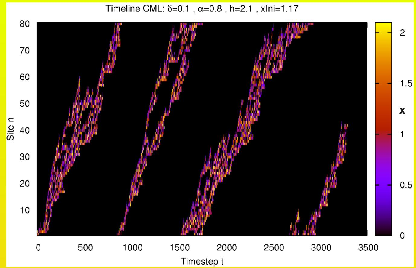
One trajectory for given initial perturbation xIni=1.17 with a lifetime of ~3300. The colour indicates the value of each site. This trajectory plays the role of a turbulent puff for the dynamical system.
