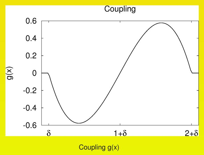
The control parameters are the height h, the coupling strength  $\alpha$  and the shift  $\delta$  (will be fixed to  $\delta=0.1$  throughout).
