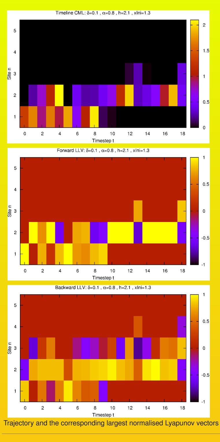
The susceptibility to perturbations of a trajectory of the CML can be infered from the linearized dynamics *M*. The growth of perturbations is governed by its singular values, i.e. it is dominated by the largest eigenvalue of  $(M^* M)$ . We wonder in what respect the corresponding eigenvectors of (M\* M) and (M M\*) characterize the most unstable directions of the forward and backwards dynamics, respectively.
