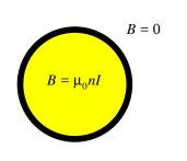
The magnetic field is ZERO outside the solenoid. Inside the solenoid, the field is
