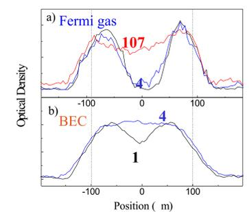
We repeat the experiment using a BEC of rubidium atoms ( $T < 0.6 T_C, N = 5 \cdot 10^4$ ). Collisions between atoms in the BEC destroy the coherent superposition of Wannier-Stark states, reducing the visibility of the interference fringes,
