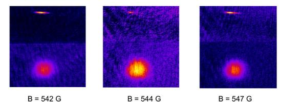
The observed losses are due to the formation of heteronuclear K-Rb molecules near the Feshbach resonance.
