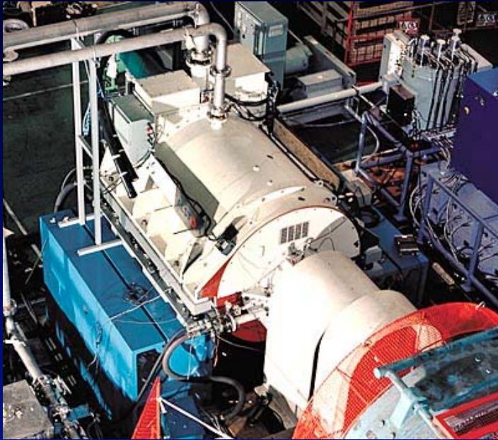
5 MW ship motor American Superconductor
