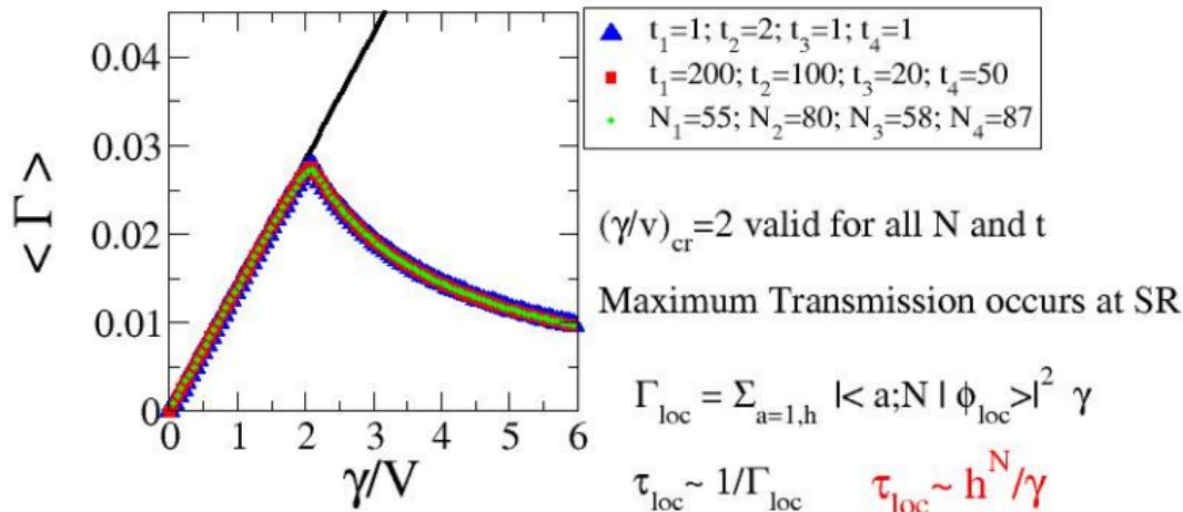
Maximum Transmission:  $T^{ab}(E=E_{loc}) = (4 t_a^2 t_b^2) / T_{tot}^2$
